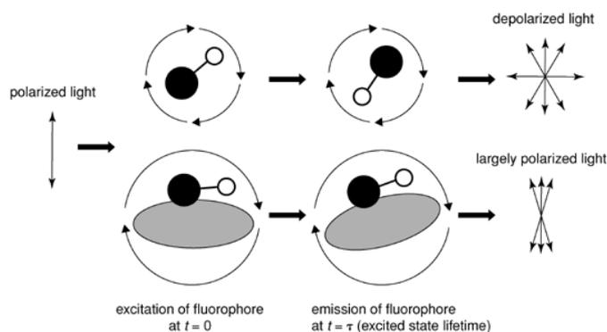
**Figure 1: Principle of fluorescence polarization.**
