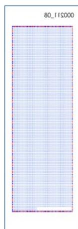
Each PEPperCHIP® Peptide Microarray is marked with microarray ID on the backside of the glass slide. The glass slide is accurately placed in an incubation tray with the microarray surface up if the microarray ID appears in the **top right corner** in a **mirror view** manner.
