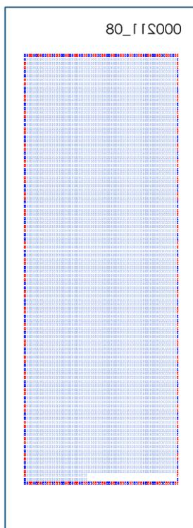
Each PEPperCHIP® Peptide Microarray is marked with microarray ID on the backside of the glass slide. The glass slide is accurately placed in an incubation tray with the microarray surface up if the microarray ID appears in the **top right corner** in a **mirror view** manner.
