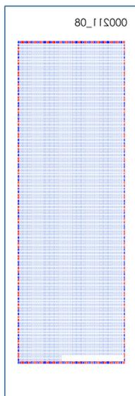
Each PEPperCHIP® Peptide Microarray is marked with microarray ID on the backside of the glass slide. The glass slide is accurately placed in an incubation tray with the microarray surface up if the microarray ID appears in the **top right corner** in a **mirror view** manner.
