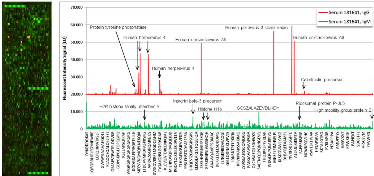
**Fig. 1:** The PEPperCHIP® Autoimmune Epitope Microarray 2.0 was assayed with human serum 181641 (1:500) followed by staining with the secondary anti-IgG (red) and anti-IgM (green) antibodies and data read-out. Simultaneous staining of the HA control peptides (green signal stretches) gave rise to the expected and well-defined spot pattern and validated the overall peptide microarray integrity and assay quality.
